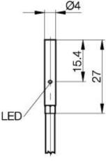
**Inductive Sensors** BES 516-3007-G-E4-C-PU-02 D4 x 27 normally-open **Sn=1,5mm** shielded
